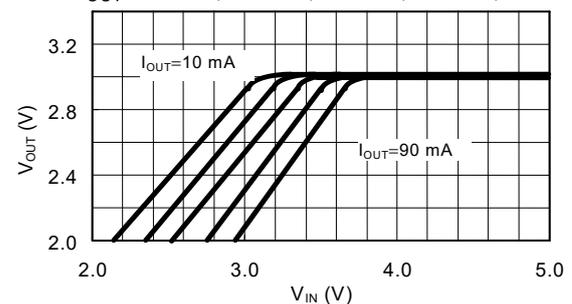
(3)  $T_a=-40^\circ\text{C}$  $I_{OUT}=10\text{ mA}, 30\text{ mA}, 50\text{ mA}, 70\text{ mA}, 90\text{ mA}$
