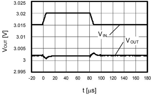
$I_{OUT} = 30 \text{ mA}$ ,  $t_r = t_f = 5.0 \mu\text{s}$ ,  $C_{OUT} = 4.7 \mu\text{F}$ ,  $C_{IN} = 0 \mu\text{F}$
