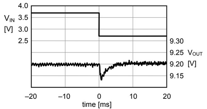
(5)  $f_{OSC} = 286\text{ kHz}$ ,  $V_{IN} = 2.7\text{ V} \rightarrow 3.7\text{ V}$
