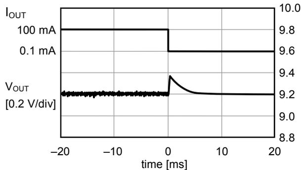
4.4 入力電圧変動 ( $V_{OUT} = 9.2\text{ V}$ ,  $I_{OUT} = 100\text{ mA}$ ,  $R_Z = 200\text{ k}\Omega$ ,  $C_Z = 0.01\text{ }\mu\text{F}$ )
