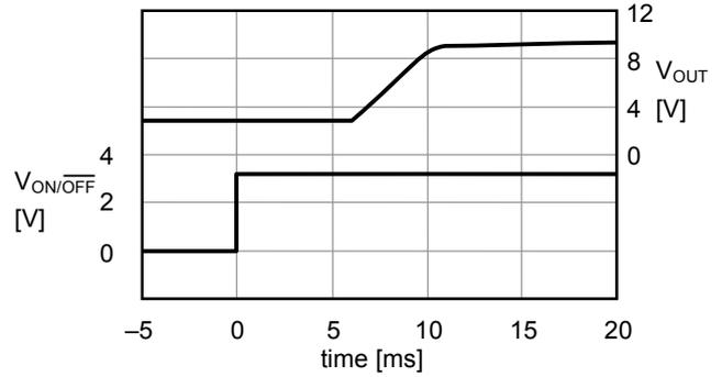
(3)  $f_{OSC} = 700\text{ kHz}$ ,  $I_{OUT} = 0\text{ mA}$ ,  $t_{SS} = 10\text{ ms}$
