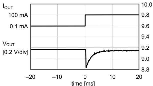
(2)  $f_{OSC} = 1133\text{ kHz}$ ,  $I_{OUT} = 100\text{ mA} \rightarrow 0.1\text{ mA}$
