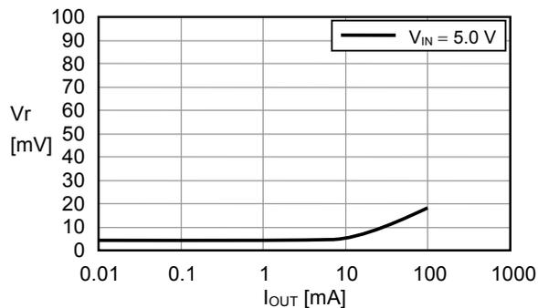
(3)  $f_{OSC} = 286 kHz$ , MaxDuty = 77 % ( $R_{OSC} = 510 k\Omega$ ,  $R_{Duty} = 750 k\Omega$ )
