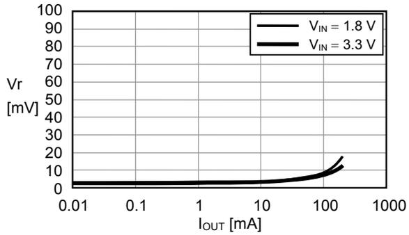
(2)  $f_{OSC} = 700\text{ kHz}$ , MaxDuty = 77 % ( $R_{OSC} = 200\text{ k}\Omega$ ,  $R_{Duty} = 300\text{ k}\Omega$ )
