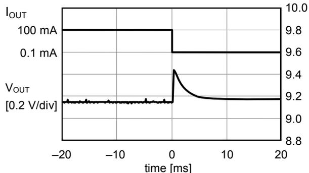
(3)  $f_{OSC} = 700\text{ kHz}$ ,  $I_{OUT} = 0.1\text{ mA} \rightarrow 100\text{ mA}$
