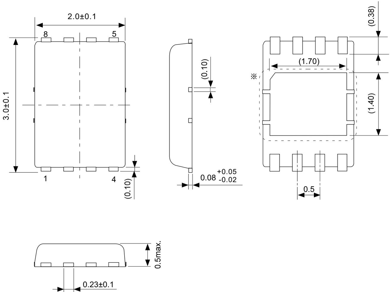
$\ast$  The heat sink of back side has different electric potential depending on the product.
