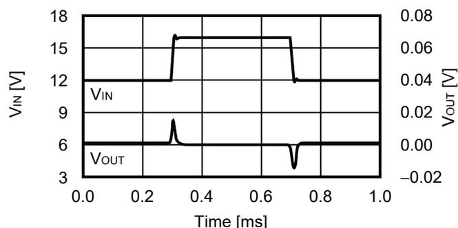
4.4 負荷変動 ( $V_{OUT} = 5.0\text{ V}$ ,  $T_a = +25^\circ\text{C}$ )
