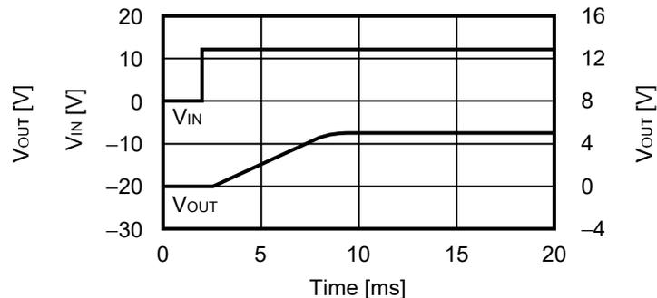
4.2 EN端子過渡応答特性 ( $V_{OUT} = 5.0\text{ V}$ ,  $V_{IN} = 12\text{ V}$ ,  $V_{EN} = 0\text{ V} \rightarrow 2.0\text{ V}$ ,  $T_a = +25^\circ\text{C}$ )
