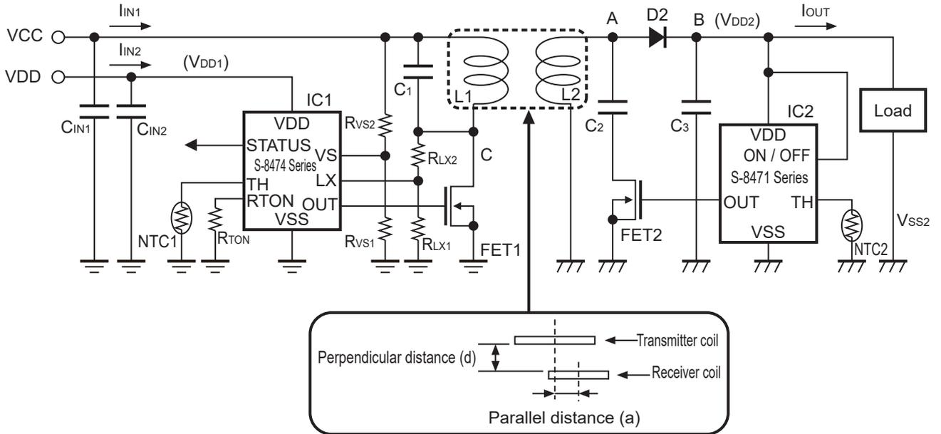
Figure 27 Evaluation Measurement Circuit Diagram
