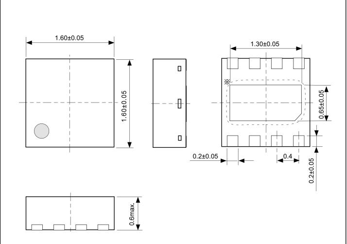
The heat sink of back side has different electric potential depending on the product.
