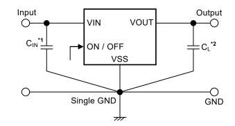
\*1. C<sub>IN</sub> is a capacitor for stabilizing the input.
