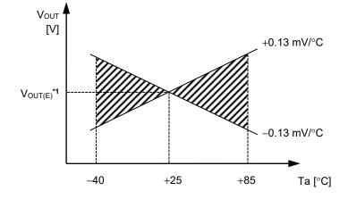
\*1.  $V_{OUT(E)}$  is the value of the output voltage measured at Ta = +25°C.
