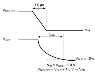
Figure 21 S-1312 Series A / B type (with discharge shunt function)
