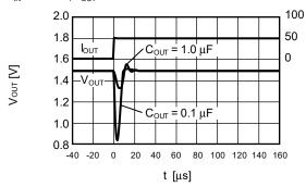
$V_{IN}$  = 2.5 V,  $I_{OUT}$  = 50 mA $\rightarrow$ 1 mA
