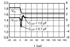
5. Load transient response characteristics — Capacity Value characteristics
