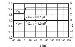
$V_{\text{IN}}$  = 4.5 V  $\rightarrow$  2.5 V,  $t_{r}$  = 5  $\mu s,~I_{\text{OUT}}$  = 50 mA
