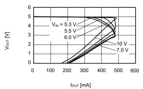
2. Output voltage vs. Input voltage
