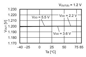
2. 5 Output voltage (V<sub>OUT</sub>) vs. Temperature (Ta)
