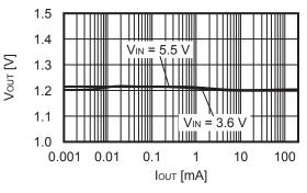
4. 2 Output voltage (VOUT) vs. Output current (IOUT)
