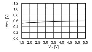
1. 17 Output voltage (VPMOUT) vs. Input voltage (VIN)
