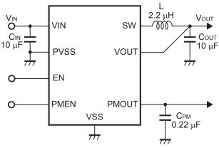
260 nA quiescent current 90.5% COT control 2.2 V to 5.5 V 0.7 V to 2.5 V, in 0.05 V step 2.6 V to 3.9 V, in 0.1 V step  $\pm 1.5\%$  (1.0 V  $\leq$  V<sub>OUT</sub>  $\leq$  3.9 V)  $\pm 15 \text{ mV} (0.7 \text{ V} \le \text{V}_{\text{OUT}} < 1.0 \text{ V})$ 1.0 MHz (at PWM operation) 420 mΩ  $320 \text{ m}\Omega$ 1 ms typ. 1.8 V typ. (detection voltage) 135°C typ. (detection temperature)
