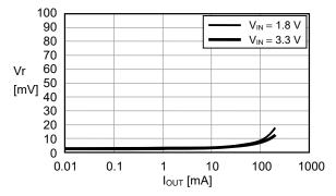
(2) fosc = 700 kHz, MaxDuty = 77 % (Rosc = 200 k $\Omega$ , R<sub>Duty</sub> = 300 k $\Omega$ )
