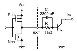
Figure 10 External Transistor Periphery
