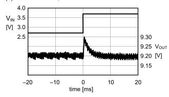
(6)  $f_{OSC} = 286 \text{ kHz}, V_{IN} = 3.7 \text{ V} \rightarrow 2.7 \text{ V}$
