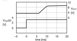
(2)  $f_{OSC} = 1133 \text{ kHz}$ ,  $I_{OUT} = 100 \text{ mA}$ ,  $t_{SS} = 10 \text{ ms}$
