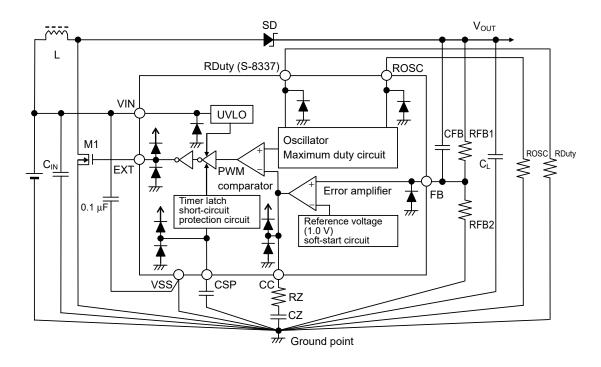
Figure 14 Standard Circuit (S-8337 Series)
