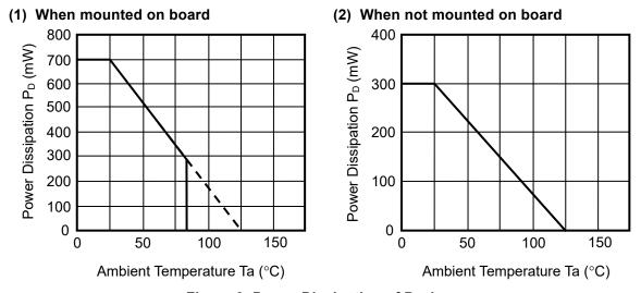
Figure 3 Power Dissipation of Package
