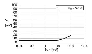
(3) fosc = 286 kHz, MaxDuty = 77 % (Rosc = 510 k $\Omega$ , R<sub>Duty</sub> = 750 k $\Omega$ )
