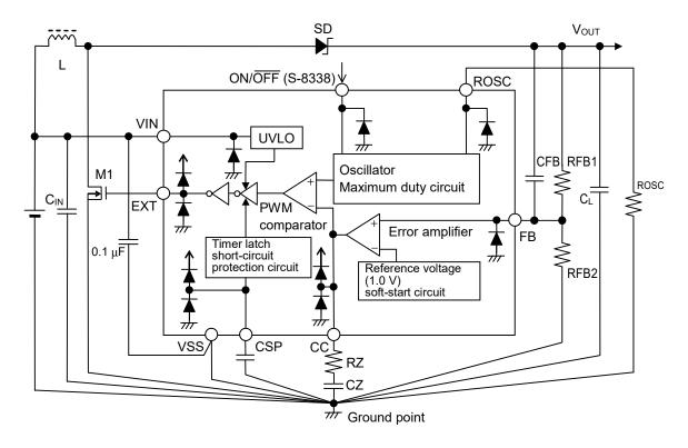
Figure 15 Standard Circuit (S-8338 Series)
