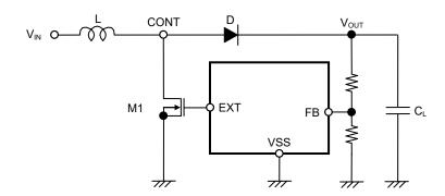
Figure 9 Step-up Switching Regulator Circuit for Basic Equations
