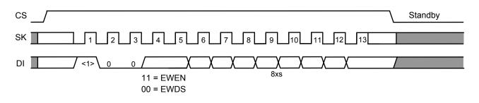
Figure 19 Write Enable / Disable Timing (S-93C76C/86C)
