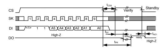
Figure 8 Data Erase Timing (S-93C46C)
