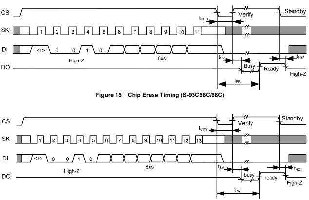
Figure 16 Chip Erase Timing (S-93C76C/86C)
