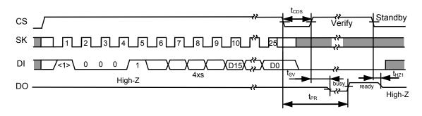
Figure 11 Chip Write Timing (S-93C46C)
