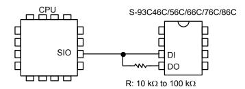
Figure 22 Connection of 3-Wire Interface
