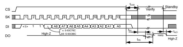
Figure 10 Data Erase Timing (S-93C76C/86C)
