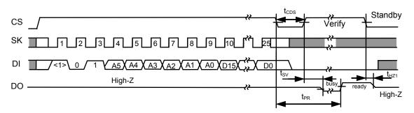
Figure 5 Data Write Timing (S-93C46C)
