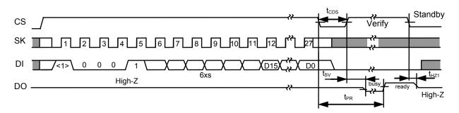
Figure 12 Chip Write Timing (S-93C56C/66C)
