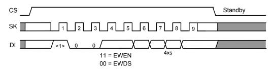
Figure 17 Write Enable / Disable Timing (S-93C46C)
