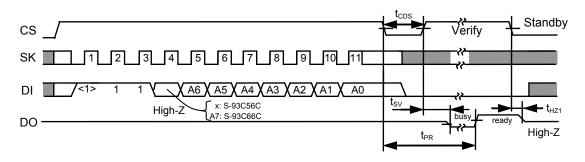
Figure 9 Data Erase Timing (S-93C56C/66C)
