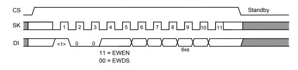
Figure 18 Write Enable / Disable Timing (S-93C56C/66C)
