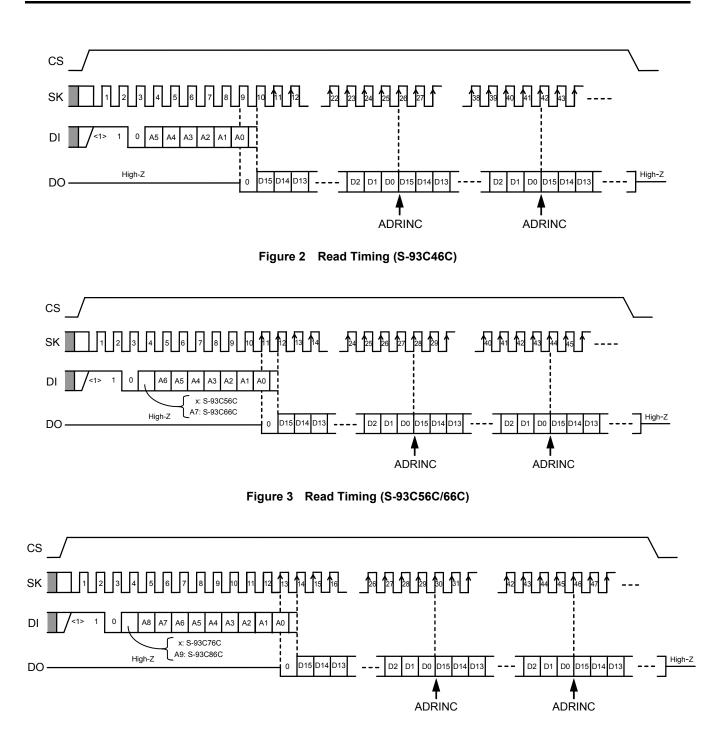
Figure 4 Read Timing (S-93C76C/86C)
