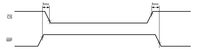
Figure 7 Invalid Timing in Write Protect
