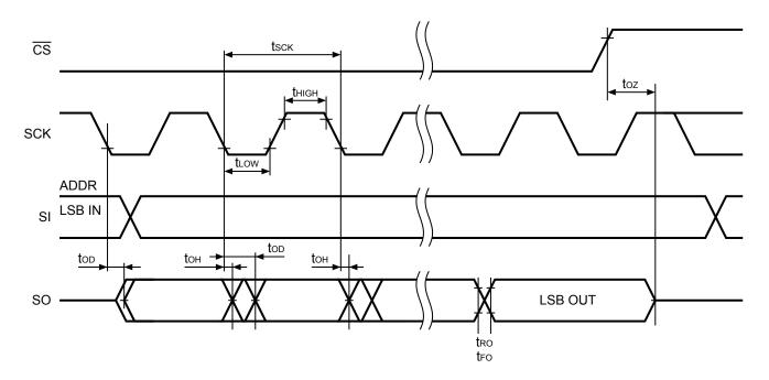
Figure 5 Serial Output Timing
