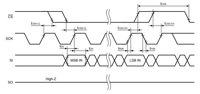
Figure 3 Serial Input Timing
