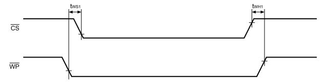
Figure 6 Valid Timing in Write Protect
