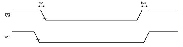
Figure 7 Valid Timing in Write Protect
