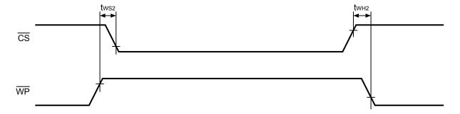
Figure 8 Invalid Timing in Write Protect
