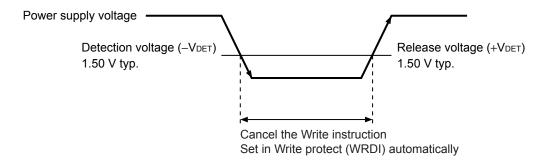
Figure 19 Operation during Low Power Supply Voltage
