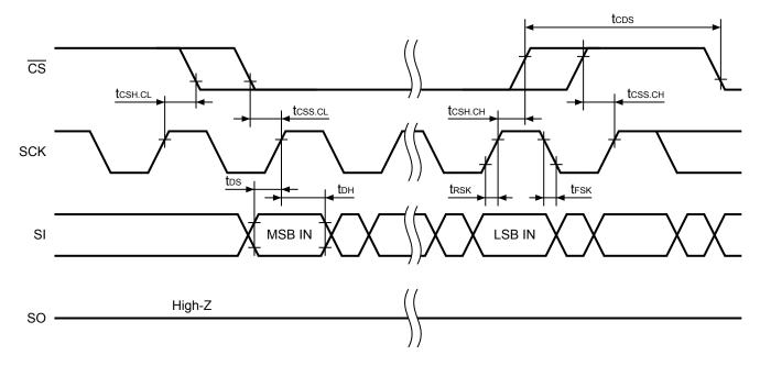
Figure 4 Serial Input Timing
