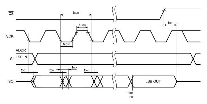
Figure 6 Serial Output Timing
