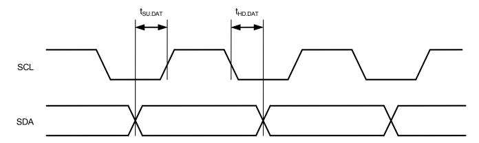
Figure 11 Data Transmission Timing
