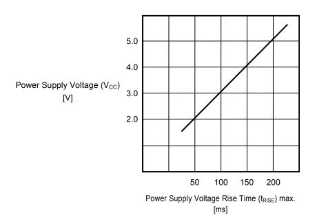
For example: If the power supply voltage = 5.0 V, raise the voltage to 5.0 V within 200 ms.
