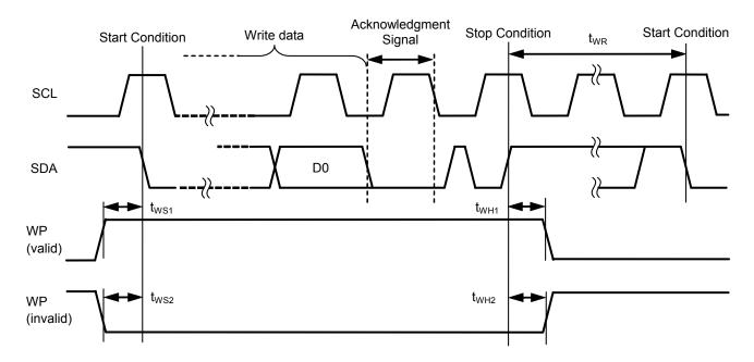
Figure 8 Write Cycle Timing
