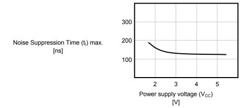
Figure 31 Noise Suppression Time for SDA and SCL Pins
