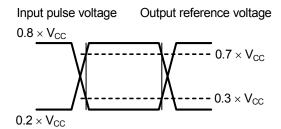
Figure 6 I/O Waveform during AC Measurement
