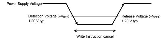
Figure 21 Operation during Low Power Supply Voltage
