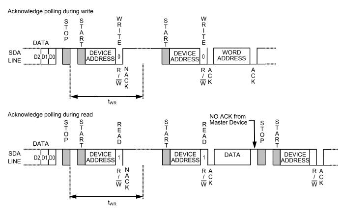
**Remark** Users are able to input word address and data after ACK output in acknowledge polling during write.
