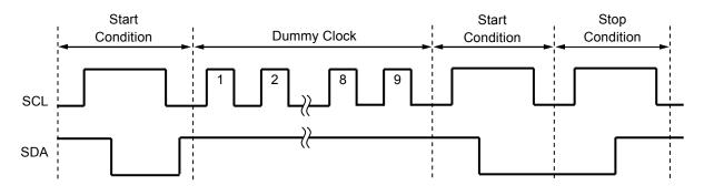
Figure 26 Resetting S-24C32C/64C
