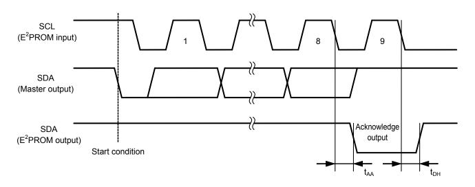
Figure 7 Acknowledge Output Timing
