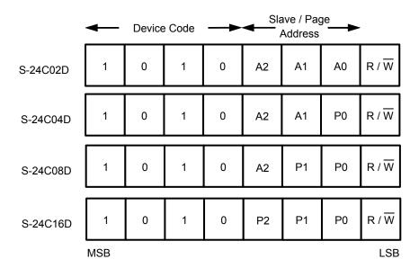
Figure 8 Device Address
