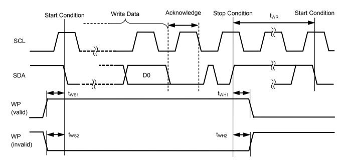
Figure 3 Write Cycle Timing
