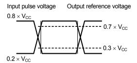
Figure 1 Input / Output Waveform during AC Measurement
