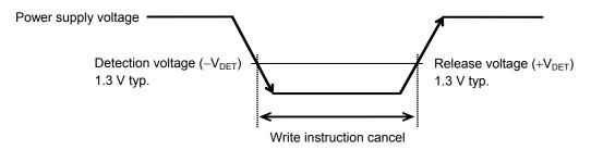
Figure 23 Operation during Low Power Supply Voltage
