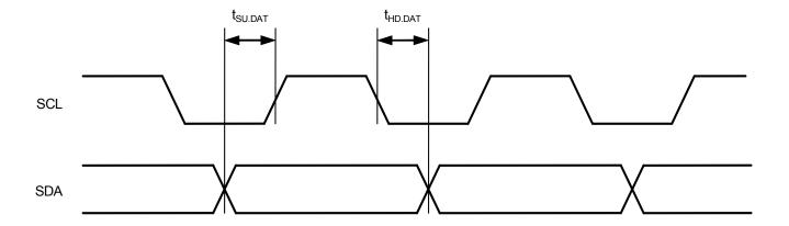
Figure 6 Data Transmission Timing
