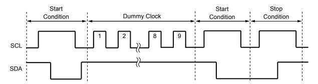
Figure 20 Resetting Method
