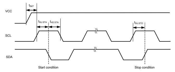
Figure 5 Start / Stop Conditions after Power-on
