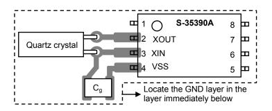
Figure 51 Connection Diagram 2
