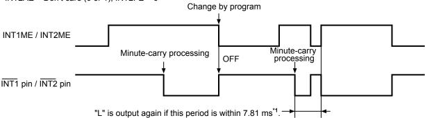
\*1. Pin output is set to "H" by disabling the output mode within 7.81 ms, because the signal of this procedure is maintained for 7.81 ms. Note that pin output is set to "L" by setting the output mode enable again.
