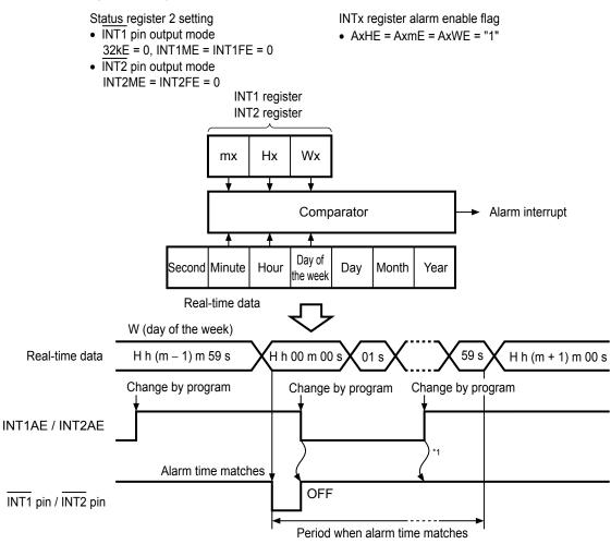
\*1. If users clear INT1AE / INT2AE once; "L" is not output from the INT1 / INT2 pin by setting INT1AE / INT2AE enable again, within a period when the alarm time matches real-time data.
