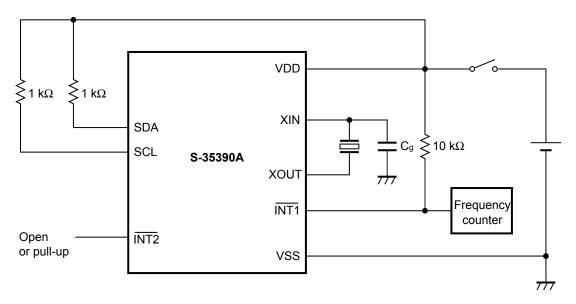
Figure 52 Configuration of Oscillation Frequency Measurement Circuit
