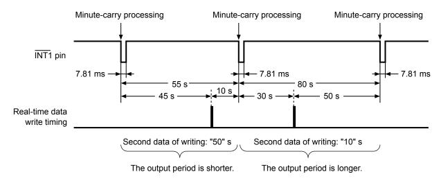
Figure 30 Timing of Minute-periodical Interrupt Output 2
