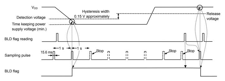
Figure 23 Timing of Low Power Supply Voltage Detection Circuit
