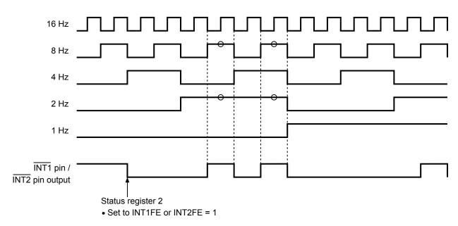
Figure 17 Example of Output from INT1 and INT2 Registers (Data Register for Output Frequency)
