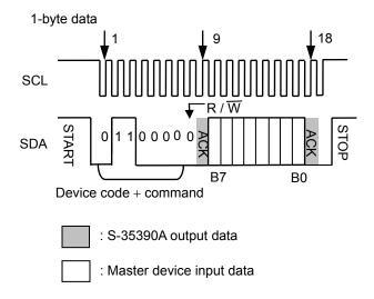
Figure 37 Example of Data Writing 1 (1-Byte Data Register)
