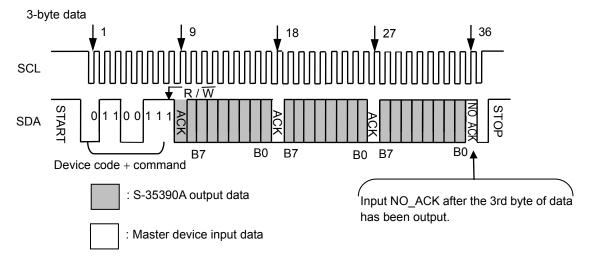
Figure 36 Example of Data Reading 2 (3-Byte Data Register)
