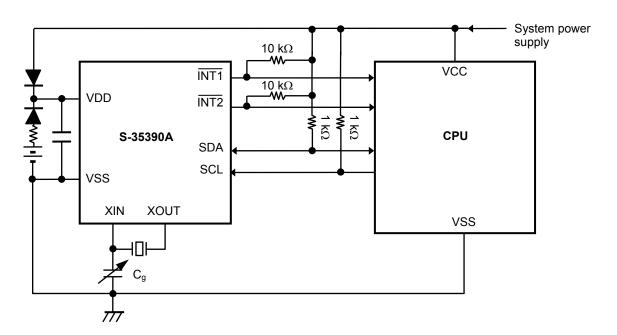
Figure 48 Application Circuit 1
