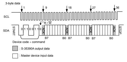
Figure 38 Example of Data Reading 2 (3-Byte Data Register)
