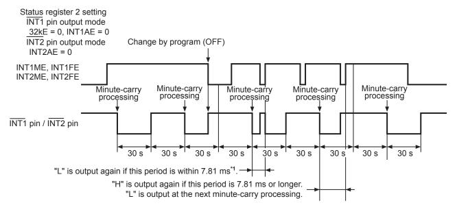
\*1. Setting the output mode disable makes the pin output "H", while the output from the  $\overline{\text{INT1}}$  /  $\overline{\text{INT2}}$  pin is in "L". Note that pin output is set to "L" by setting the output mode enable again.
