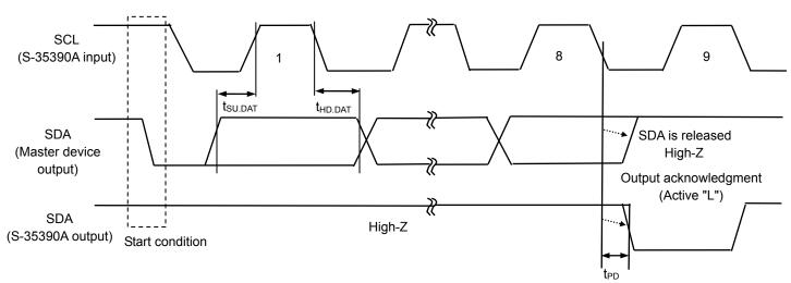
Figure 34 Output Timing of Acknowledgment Signal
