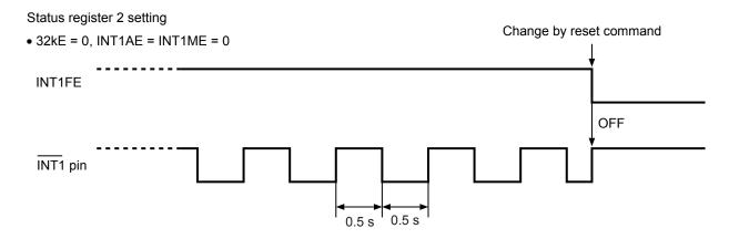
Figure 31 Output Timing of INT1 Pin during Operation of Power-on Detection Circuit
