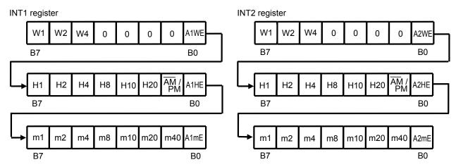
Figure 14 INT1 Register and INT2 Register (Alarm-Time Data)
