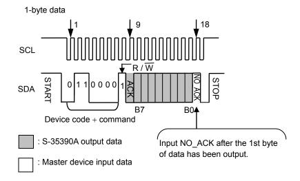
Figure 35 Example of Data Reading 1 (1-Byte Data Register)
