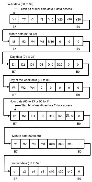
Figure 11 Real-Time Data Register
