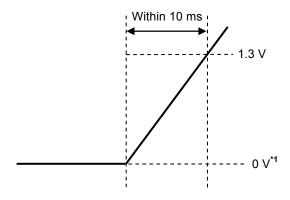
\*1. 0 V indicates that there are no potential differences between the VDD pin and VSS pin of S-35390A.
