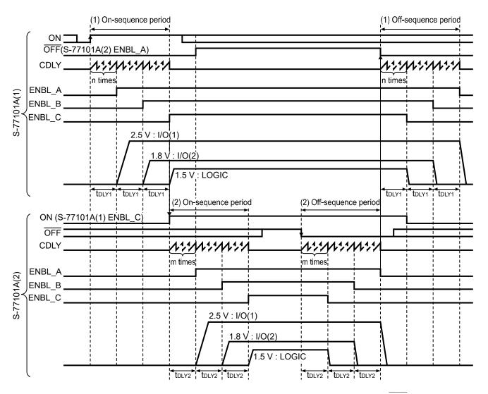
Figure 14 Timing Chart at Cascade Connection (S-77101A: Reverse Type, with OFF pin)
