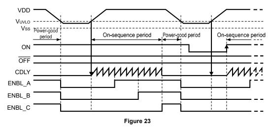
(2) When low voltage is detected during on-sequence period and off-sequence period
