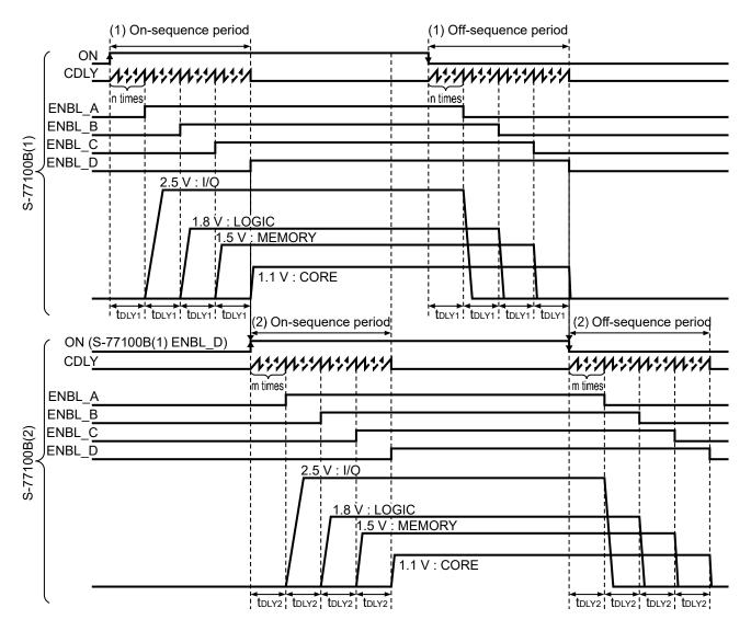
Figure 12 Timing Chart at Cascade Connection (S-77100B: Forward Type)
