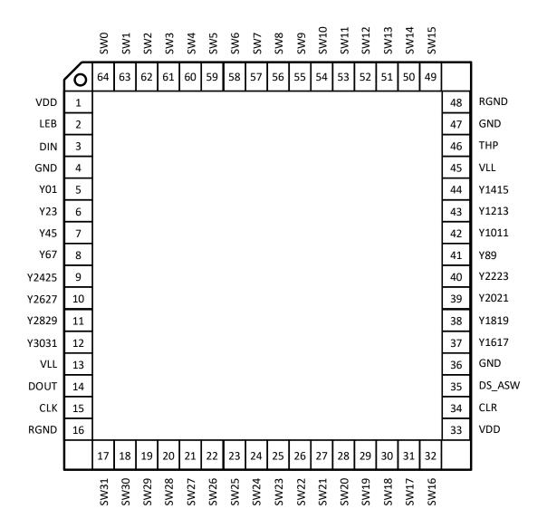
Fig.5 Pin Configuration
