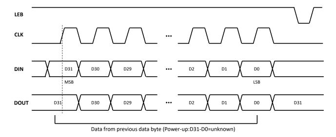
Fig.4 Latch Enable Interface Timing
