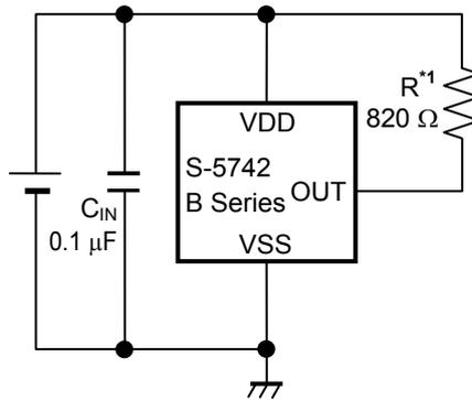
\*1. Resistor (R) is unnecessary for Nch driver + built-in pull-up resistor product.
