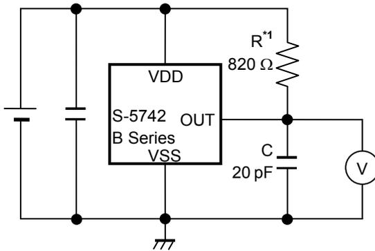
\*1. Resistor (R) is unnecessary for Nch driver + built-in pull-up resistor product.
