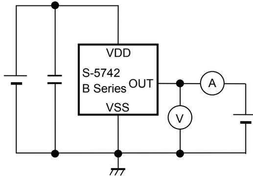
**Figure 7 Test Circuit 3**
