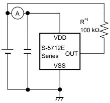
\*1. Resistor (R) is unnecessary for the CMOS output product.
