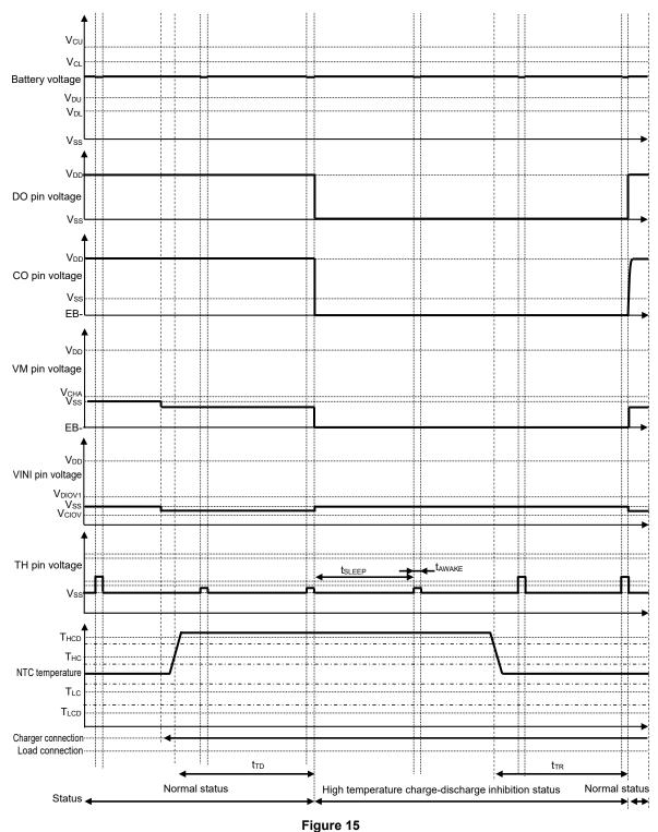
Remark 1. Figure 15 shows a time chart when N = 2 and the temperature of an NTC thermistor changes from below
