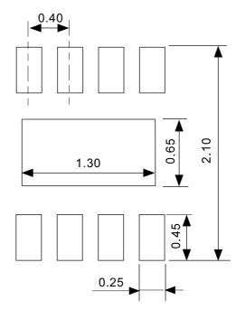
Caution It is recommended to solder the heat sink to a board in order to ensure the heat radiation.
