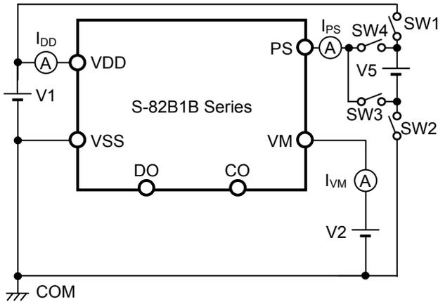
Figure 6 Test Circuit 3
