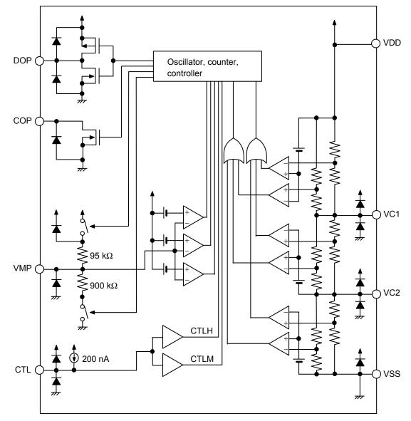
Remark All diodes shown in figure are parasitic diodes.
