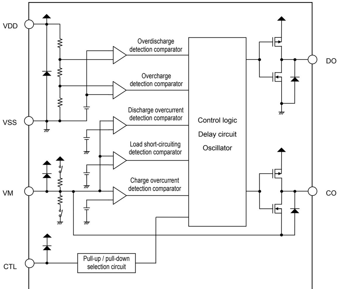
**Remark** All the diodes shown in the figure are parasitic diodes.
