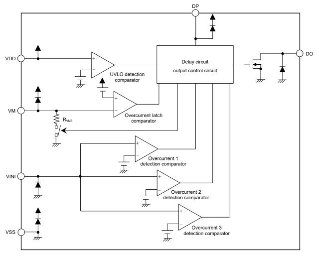
Remark All the diodes shown in the figure are parasitic diodes.
