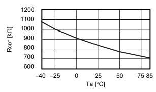
3. 4  $V_{CDT}$  vs Ta ( $V_{DS} = 15.5 \text{ V}$ )
