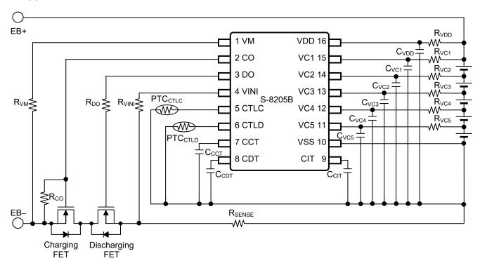
Figure 15 Overheat Protection via PTC
