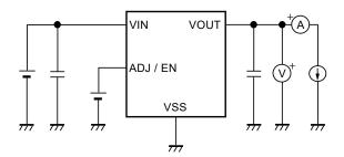
Figure 5 Test Circuit 2
