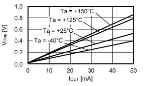
5. Dropout voltage vs. Junction temperature
