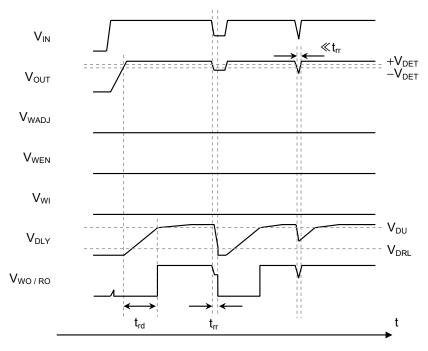
Figure 41 Example of Detector Operation
