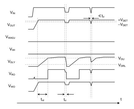
Figure 43 Example of Detector Operation
