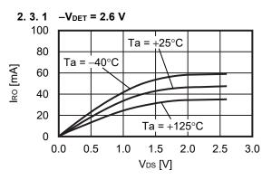
2.4 Reset output current vs. Output voltage
