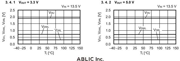
3. 5 Watchdog activation threshold current, watchdog deactivation threshold current vs. Junction temperature
