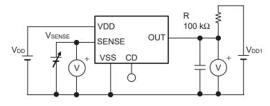
Figure 25 Test Circuit of Response Time
