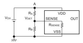
Figure 18 Detection Voltage External Setting Circuit
