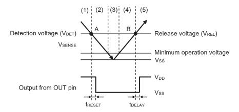
**Remark** The release voltage is set to the same value as the detection voltage, since there is no hysteresis width.
