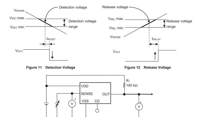
Figure 13 Test Circuit of Detection Voltage and Release Voltage
