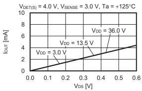
Remark V<sub>DS</sub>: Drain-to-source voltage of the output transistor
