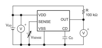
Figure 29 Test Circuit of Release Delay Time
