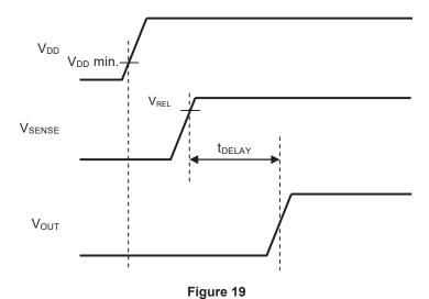
Caution When the SENSE pin is turned on before the VDD pin, a release may mistakenly occur even if  $V_{\text{SENSE}}$  is less than  $V_{\text{REL}}$ .
