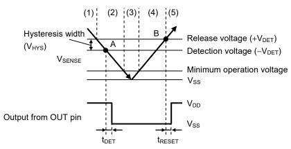
Figure 23 Timing Chart of S-19104/19106 Series C Type
