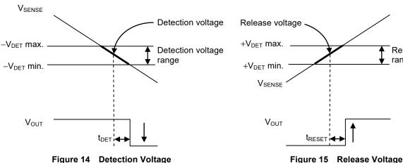
Figure 14 Detection Voltage
