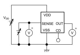
Figure 6 Test Circuit 1 (CMOS output product)
