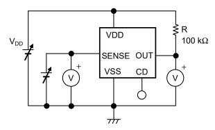
Figure 5 Test Circuit 1 (Nch open-drain output product)
