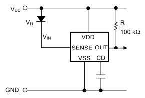
Figure 40 Detection voltage change when using a diode (Nch open-drain output product)
