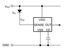
Figure 41 Detection voltage change when using a diode (CMOS output product)
