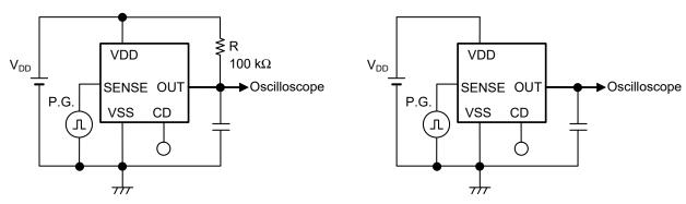
Figure 31 Test Circuit of Response Time (Nch open-drain output product)
