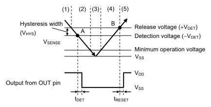
Figure 21 Timing Chart of S-19104/19106 Series N Type
