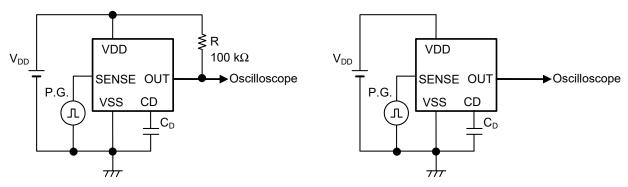
Figure 34 Test Circuit of Release Delay Time (Nch open-drain output product)
