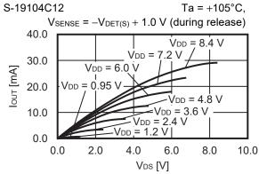
Remark V<sub>DS</sub>: Drain-to-source voltage of the output transistor
