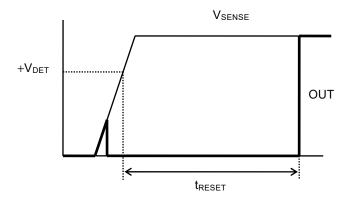
Figure 18 Release Delay Time
