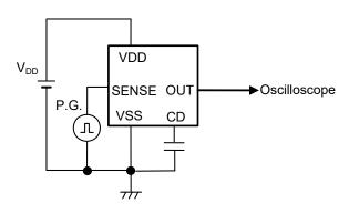
Figure 10 Test Circuit 4 (CMOS output product)
