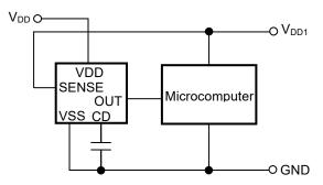
Figure 37 Example of Reset Circuit (CMOS output product)
