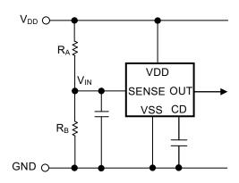
Figure 39 Detection voltage change when using a resistance divider (CMOS output product)
