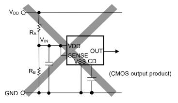
Figure 19 Example for Bad Implementation Due to Detection Voltage Change
