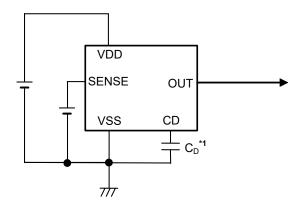
\*1. The delay capacitor (CD) should be connected directly to the CD pin and the VSS pin.
