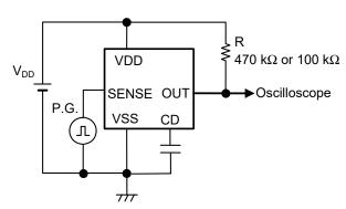
Figure 9 Test Circuit 4 (Nch open-drain output product)
