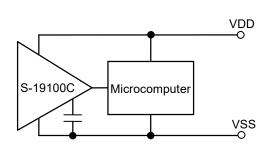
Figure 26 Example of Reset Circuit (CMOS Output Product)
