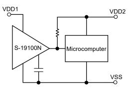
Figure 27 Example of Reset Circuit (Nch Open-drain Output Product)
