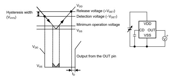
**Remark** When  $V_{DD}$  is the minimum operation voltage or less, the output voltage from the OUT pin is indefinite in the shaded area.
