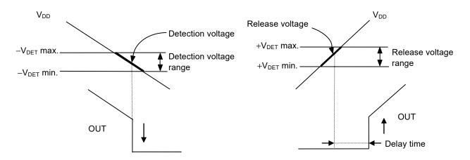
Figure 17 Detection Voltage
