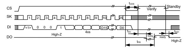
Figure 11 Chip Write Timing (S-93A46B)
