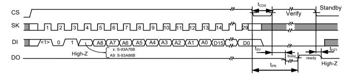
Figure 7 Data Write Timing (S-93A76B/86B)
