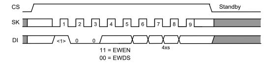
Figure 17 Write Enable / Disable Timing (S-93A46B)
