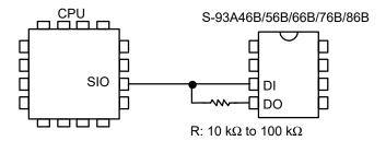
Figure 22 Connection of 3-Wire Interface
