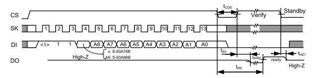
Figure 10 Data Erase Timing (S-93A76B/86B)
