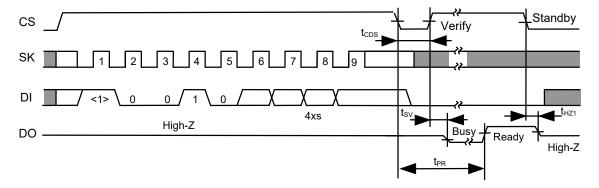
Figure 14 Chip Erase Timing (S-93A46B)
