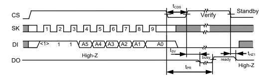
Figure 8 Data Erase Timing (S-93A46B)
