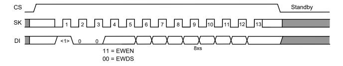
Figure 19 Write Enable / Disable Timing (S-93A76B/86B)
