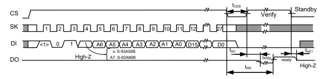
Figure 6 Data Write Timing (S-93A56B/66B)
