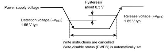
Figure 20 Operation during the Low Power Supply Voltage
