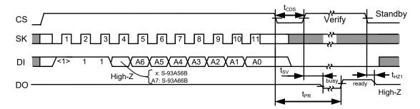
Figure 9 Data Erase Timing (S-93A56B/66B)
