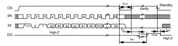
Figure 5 Data Write Timing (S-93A46B)
