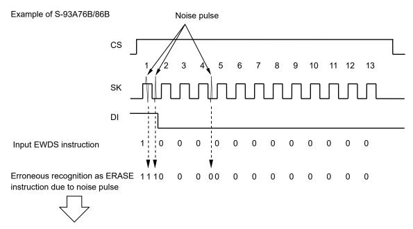
In products that do not incorporate a clock pulse monitoring circuit, "FFFFh" is mistakenly written to address 00h. However the S-93A76B/86B detects the overcount and cancels the instruction without performing a write operation.
