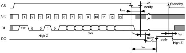
Figure 16 Chip Erase Timing (S-93A76B/86B)
