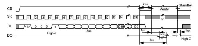
Figure 13 Chip Write Timing (S-93A76B/86B)
