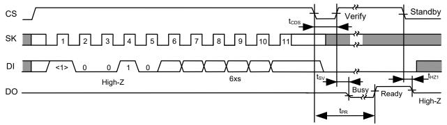
Figure 15 Chip Erase Timing (S-93A56B/66B)
