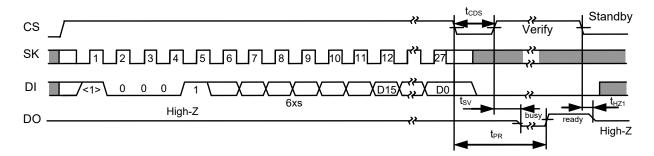
Figure 12 Chip Write Timing (S-93A56B/66B)
