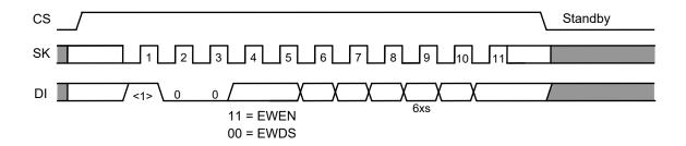
Figure 18 Write Enable / Disable Timing (S-93A56B/66B)
