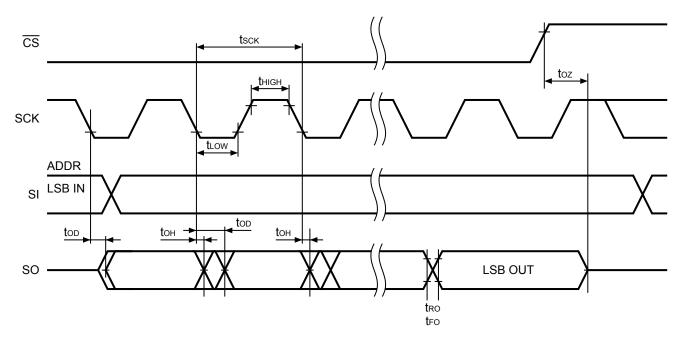
Figure 7 Serial Output Timing
