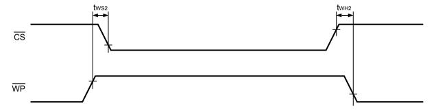
Figure 9 Invalid Timing in Write Protect
