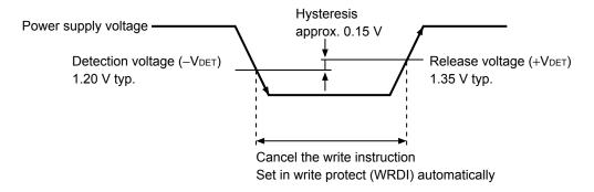
Figure 20 Operation during the Low Power Supply Voltage (S-25A080A/160A/320A)
