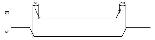
Figure 8 Valid Timing in Write Protect
