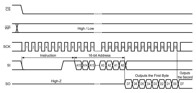
Remark In the S-25A080A and the S-25A080B, the higher addresses A15 to A10 = Don't care. In the S-25A160A and the S-25A160B, the higher addresses A15 to A11 = Don't care. In the S-25A320A and the S-25A320B, the higher addresses A15 to A12 = Don't care.
