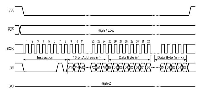
**Remark** In the S-25A080A and the S-25A080B, the higher addresses A15 to A10 = Don't care. In the S-25A160A and the S-25A160B, the higher addresses A15 to A11 = Don't care. In the S-25A320A and the S-25A320B, the higher addresses A15 to A12 = Don't care.
