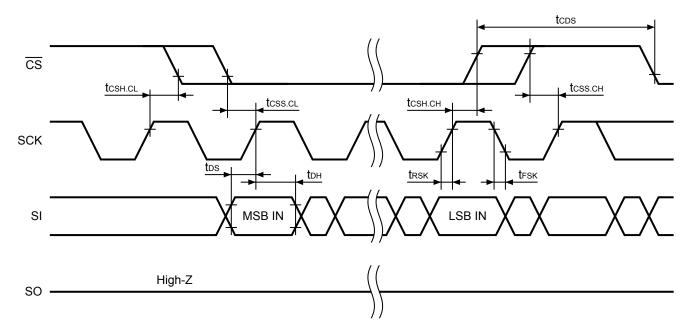
Figure 5 Serial Input Timing
