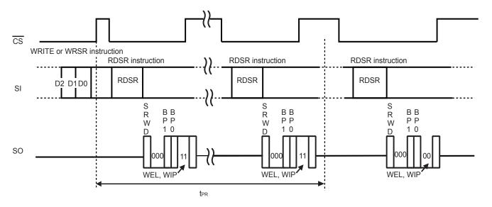
Figure 11 Usage Example of WEL, WIP Bits during Write
