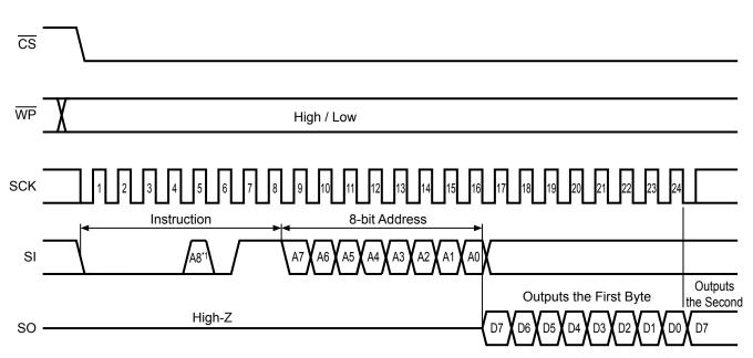
\*1 In the S-25A040A, assign bit A8 in the address into the fifth bit in an instruction code.
