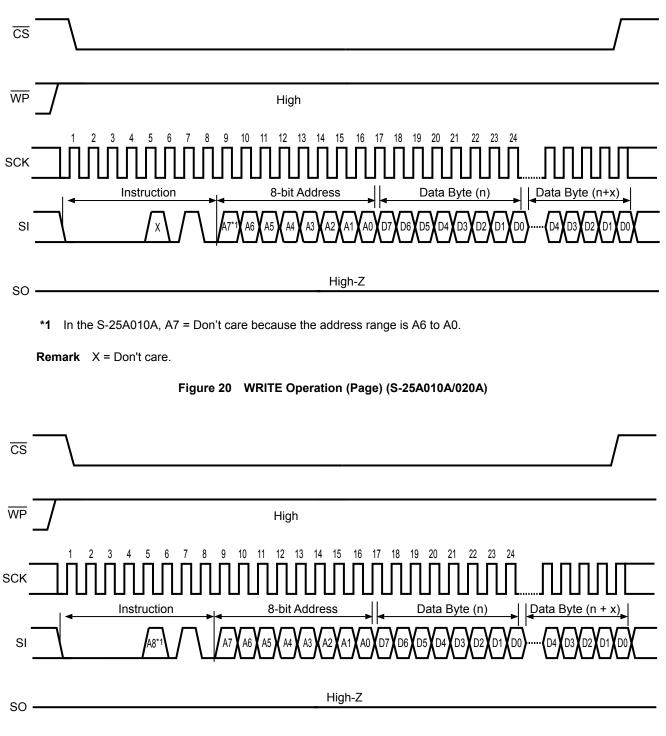
\*1 In the S-25A040A, assign bit A8 in the address into the fifth bit in an instruction code.
