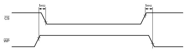
Figure 9 Invalid Timing in Write Protect
