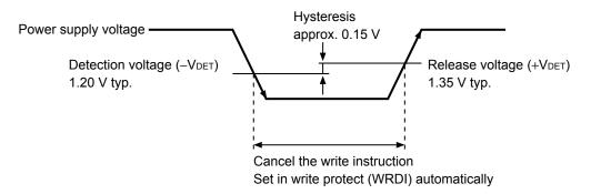
Figure 23 Operation during the Low Power Supply Voltage
