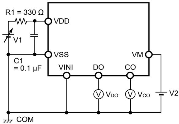
**Figure 3 Test Circuit 1**
