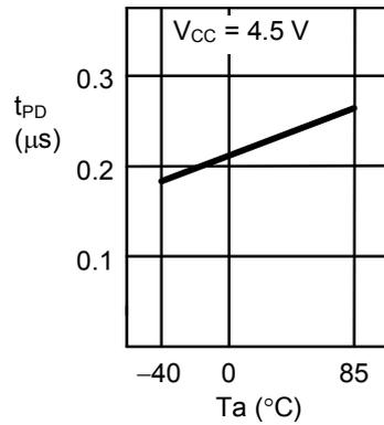
2.7 数据输出延迟时间 $t_{PD}$ —周围温度 $T_a$
