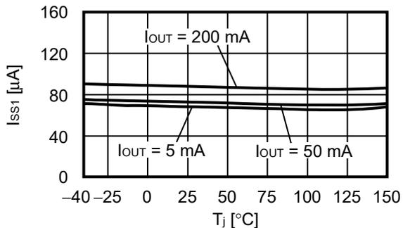
3.3.2  $V_{OUT} = 5.0\text{ V}$ ,  $-V_{DET} = 4.7\text{ V}$
