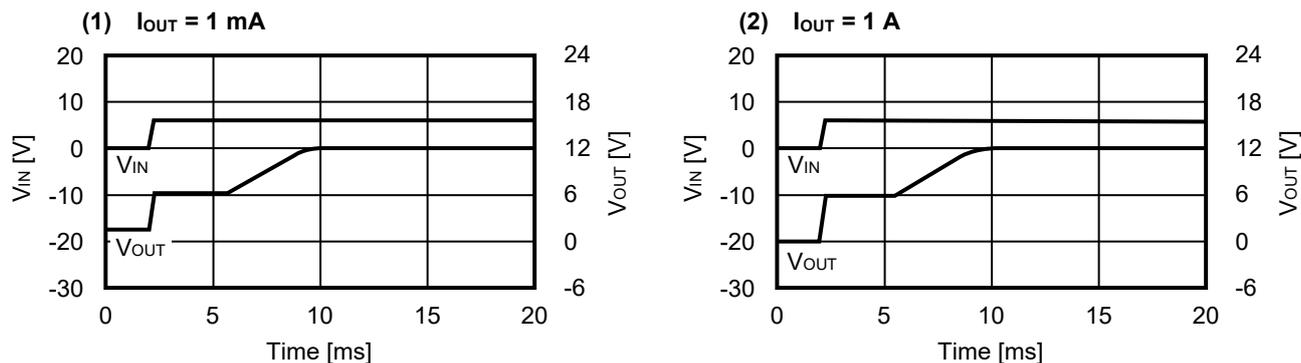
4.2 EN端子过渡响应特性 ( $V_{OUT} = 12\text{ V}$ ,  $V_{IN} = 6\text{ V}$ ,  $V_{EN} = 0\text{ V} \rightarrow 2.0\text{ V}$ ,  $T_a = +25^\circ\text{C}$ )
