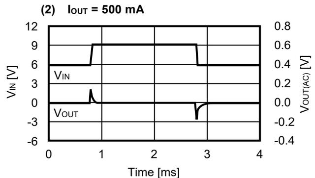
4.4 负载过渡响应 ( $V_{OUT} = 12\text{ V}$ ,  $V_{IN} = 6\text{ V}$ ,  $T_a = +25^\circ\text{C}$ )
