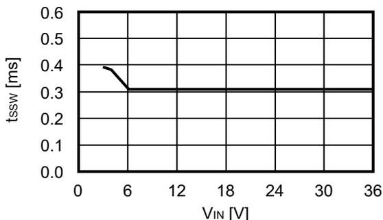
1.7 软启动时间 ( $t_{SS}$ ) – 输入电压 ( $V_{IN}$ )
